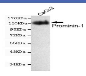
Western blot detection of Prominin-1 in CaCo2 cell lysate using Prominin-1 mouse mAb (1:1000 diluted).Predicted band size:97KDa.Observed band size:133KDa
