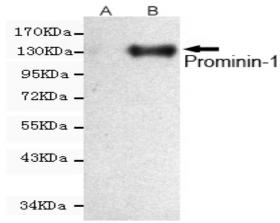
Western blot detection of Prominin-1 expression in CHO-k1 cells non-transfected (A) or transfected (B) with Prominin-1 and using Prominin-1 mouse mAb (1:1000 diluted). Predicted band size:97KDa. Observed band size:133KDa.
