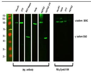
Western Blot analysis of various cells using primary antibody diluted at 1:1000(4°C overnight). Secondary antibody:Goat Antirabbit IgG IRDye 800( diluted at 1:5000, 25°C, 1 hour)
