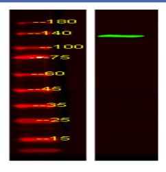
Western Blot analysis of HEK293 lysis, using primary antibody at 1:1000 dilution. Secondary antibody(catalog#:RS23920) was diluted at 1:10000
